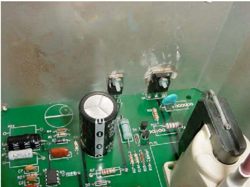
Solder the red wire from your old connector to the yellow wire on the new hIV board. Solder the white wire on your old connector to the black wire on the new HV board. Cover with some electrical tape or heat shrink tubing.
