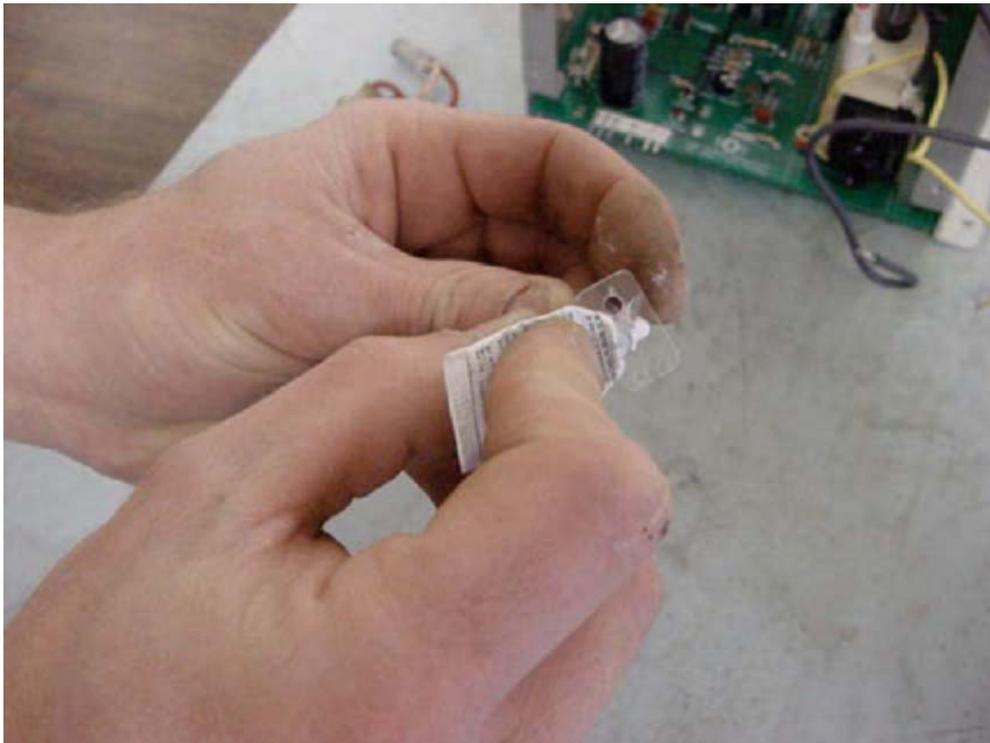
Place the mica insulators on your aluminum HV cage. Be sure to line up the holes in the insulators with the holes you made in the HV cage.
